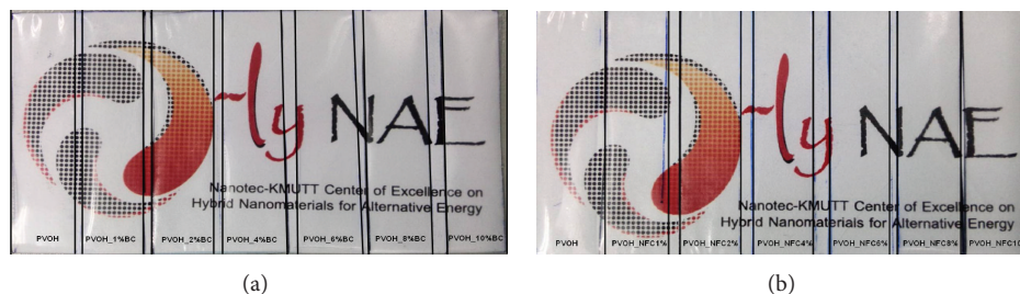
FIGURE 12: Photographs showing transparency of the PVA/cellulose nanofiber composite films; PVA/BC (a) and PVA/NFC (b).
