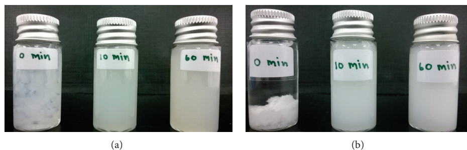
FIGURE 1: Photographs of BC fibers (a) and NFC fibers (b) both before (left bottles) and after experienced mechanical treatment for 60 min (right bottles).
