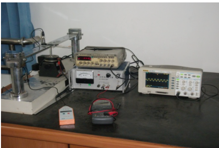
FIGURE 9: Experimental platform of piezoelectric generator.
