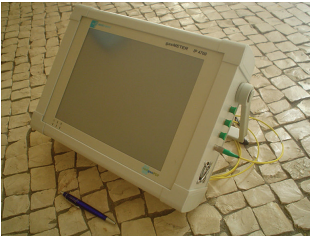
FIGURE 12: (a) Diagram of the gas measurement unit prototype; (b) photo of the unit; (c) response for a methane concentration change.
