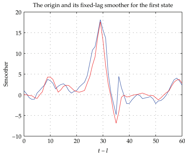
Figure 5: The origin and its fixed-lag smoother \hat{x}_1(t-l | t) , where the blue line is the origin signal, the red line is the smoother.
