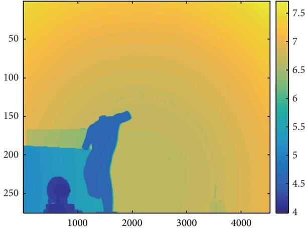
FIGURE 8: Laboratory distance image. The scene distances range from 3.9 to 7.7 meters.
