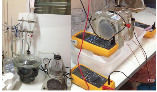
FIGURE 1: The RCPT test setup with ASTM C1202 [11].
