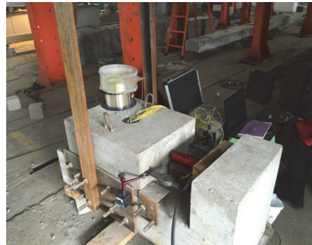
(b) Photo of the shearing tests
