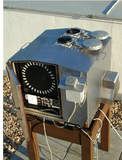
FIGURE 6: The automated EN sky patrol photographic camera operated by the Ondrejov Observatory, Department of Interstellar Matter.
