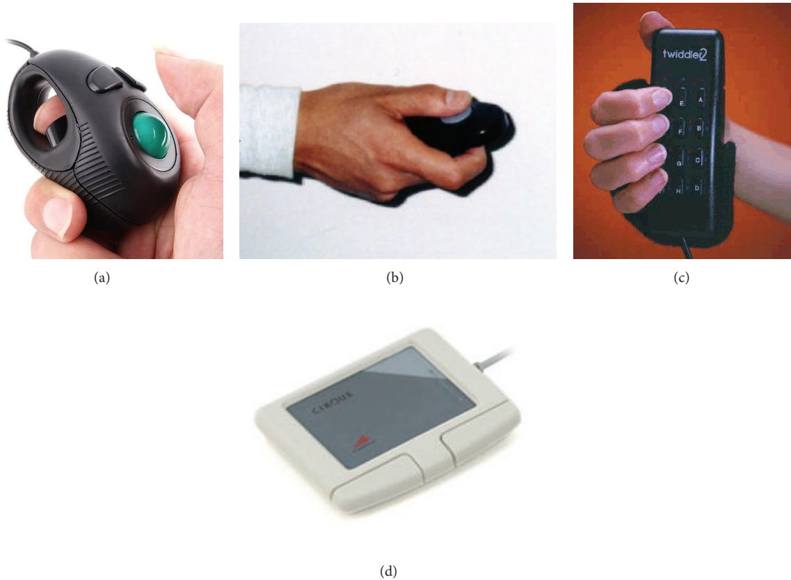
FIGURE 1: Adaptations of traditional pointing devices. (a) The 4D Off-Table Hand Track mouse , (b) the RemotePoint , (c) the Twiddler2 , and (d) the EasyCat Touchpad . (a)–(d) from [14, 25–27], respectively.
