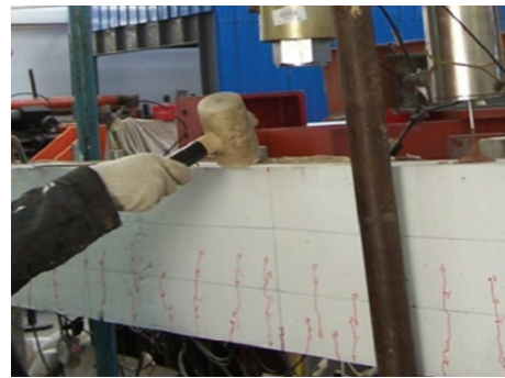
FIGURE 9: Hammer load of simple-supported beam.
