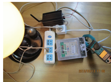
FIGURE 12: ZBEMCS, standard wattmeter, and clamp meter.
