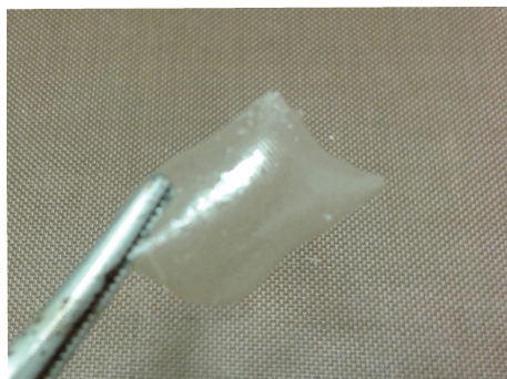
FIGURE 4: The visual appearance of films produced with HCl as catalyst agent.
