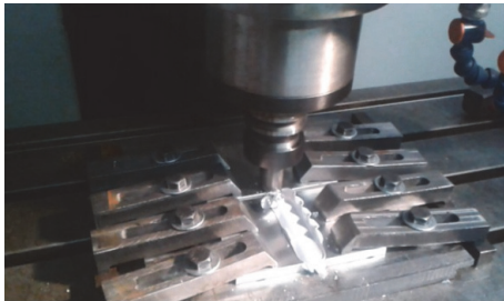
FIGURE 3: The two welding plates clamped to machine bed and the welding tool at the end of the FSW process.
