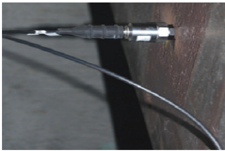
FIGURE 2: Typical accelerometer attachment.
