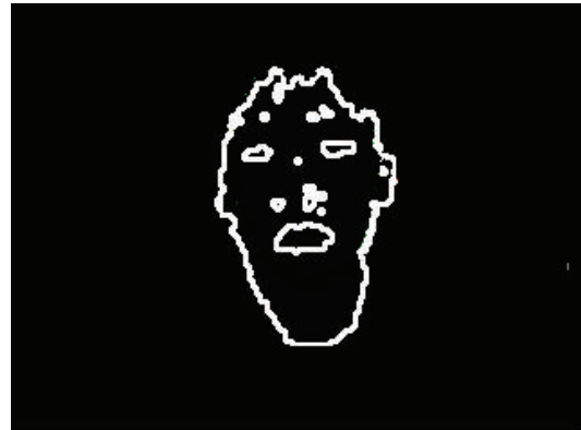
FIGURE 3: The result of the Sobel edge detection.
