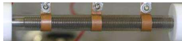
(b) Electrode spaces of 4cm
