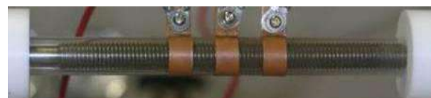
(a) Electrode spaces of 1cm
