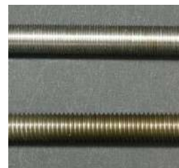
Figure 2. Different screw electrodes of the screw thread interval (1.00mm or 1.75mm).
