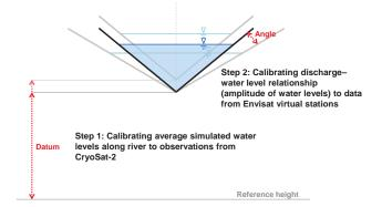
**Figure 4.** Sketch of the two-step cross-section calibration with their calibration parameters.
