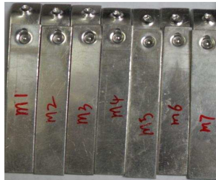
(b) Failed SPR joints
