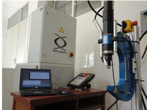
Fig. 5. Test set up of process window monitoring of SPR process
