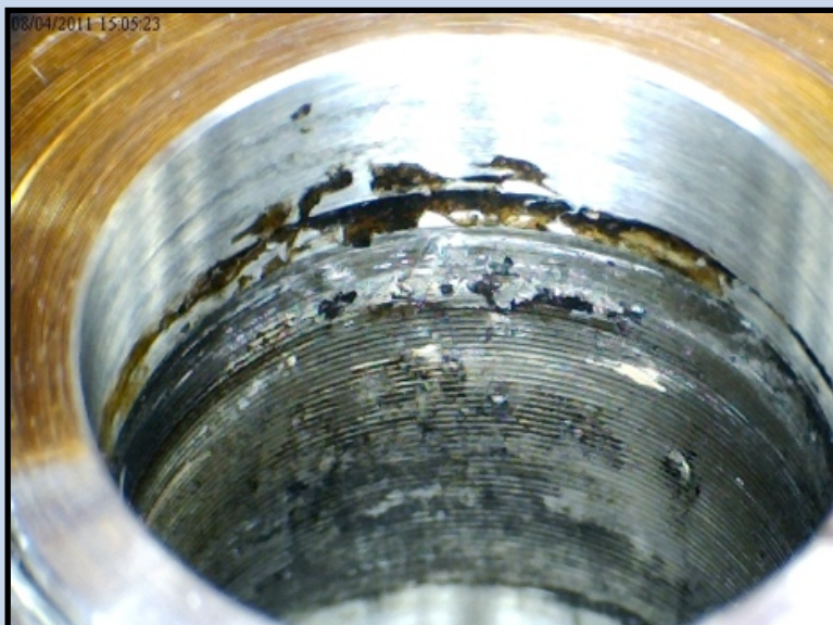
Large amount of discolouration and black deposits on head taper
