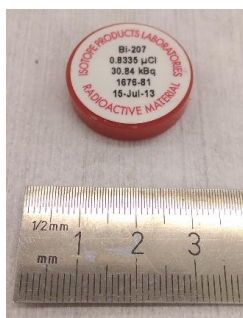
Figure 6: ^{207}\text{Bi} certified source.
