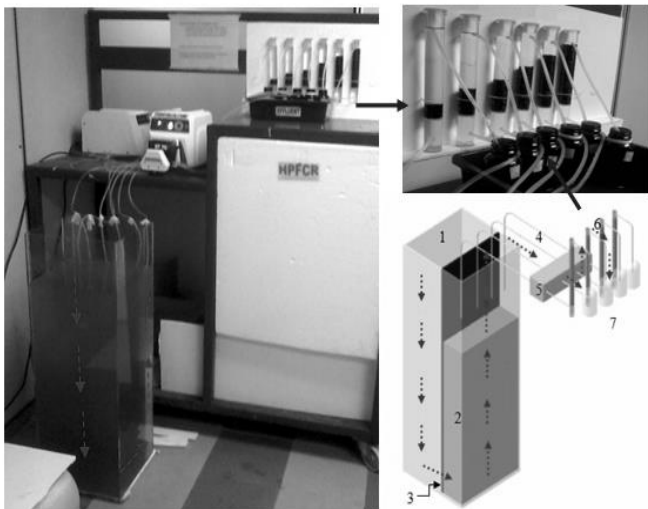
Figure.1. Hybrid plug-flow column reactor configuration; (1) Influent tank (2) Sand Filter (3) Perforated Holes with 2mm di-
