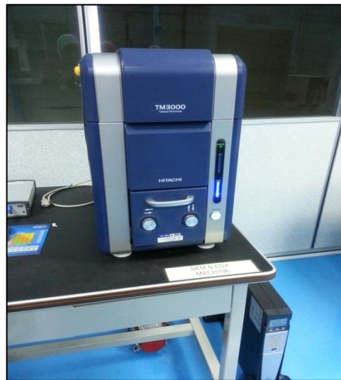
Figure 4.3: SEM with EDX: TM3000 Hitachi at UniMAP
