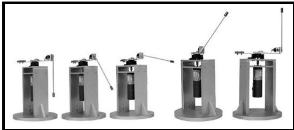
Figure 2. 5: A Rotary Inverted Pendulum Type.
