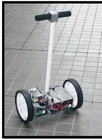
Figure 2. 4: Mobile Inverted Pendulum Type.
