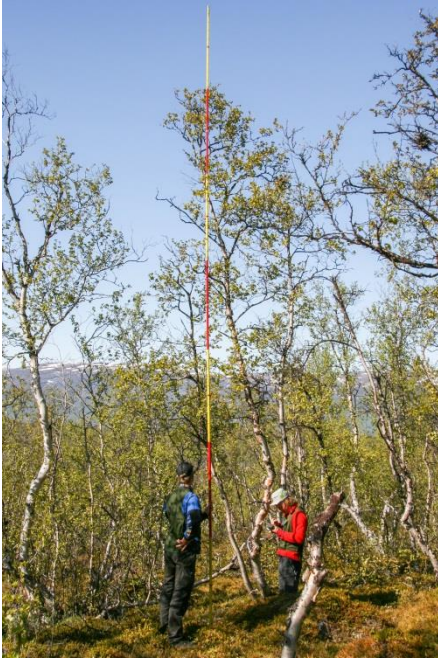
Figure 2. Paper I, measuring height of a mountain birch using a 7 m measuring pole.
