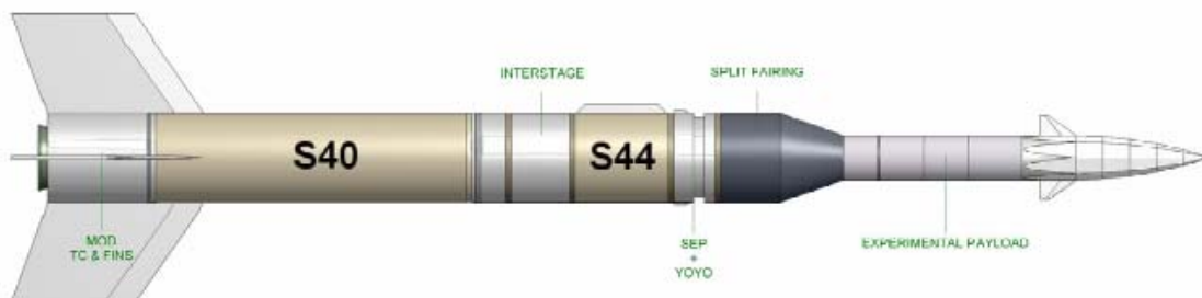
Figure 2: S 40 Launcher system for SHEFEX II and payload configuration
