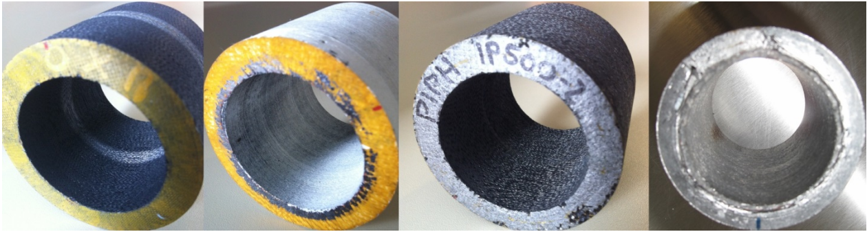
Figure 13: Demonstration of damage free (at \tau = 6.72\% ) operated cylindrical CMC segments, after WS1-A.
