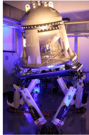
Figure 9: CTD mounted on Hexapod System
