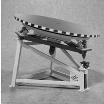
Figure 7: Sketch of the Tilt Table equipped with the Turn Table
