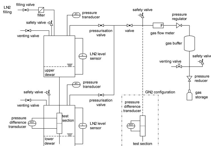
Figure 5: Sketch of the LN<sub>2</sub>/GN<sub>2</sub> experiment setup.
