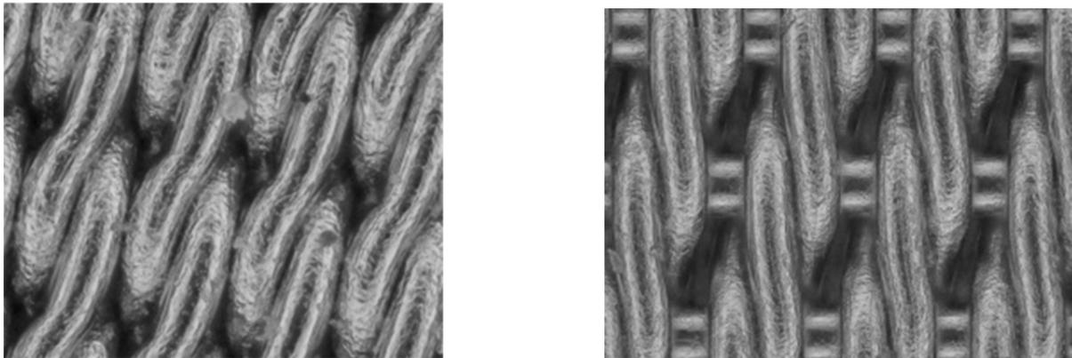
Figure 1: Comparison of DTW 200x1400 (left) and BM 165x800 (right) weave.
