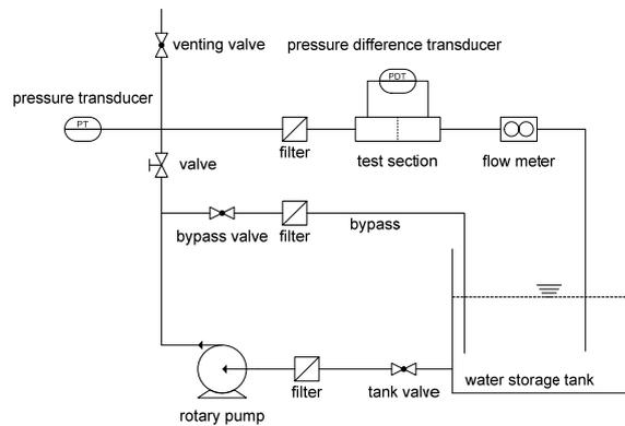
Figure 4: Sketch of the experiment setup for water tests.
