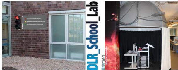
Figure 5 Left image: at the entrance wall of the DLR Institute of Space Systems in Bremen a space weather traffic signal automatically visualize by means of GMDN anisotropy data the CME location between Sun and Earth. Right image: planetarium dome with fish eye lenses, laser beamer and PC for real time visualization of cosmic ray shower by means of the two layers of plastic scintillator detectors and photomultiplier tubes (in the upper right part of the image).
