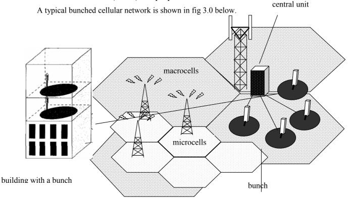
Fig 3.0 A Scenario of mixed cell structure with Bunched Network
