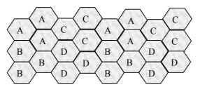
Fig 2.0 MTN (Nigeria) 4 X 3 Frequency Reuse Pattern.
