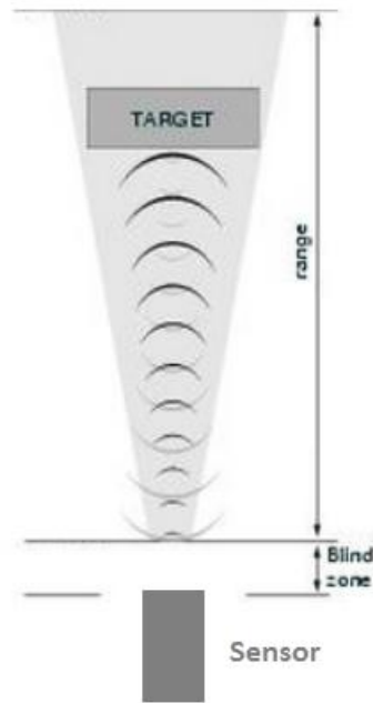
Figure 2: Ultrasonic sensor operation.
