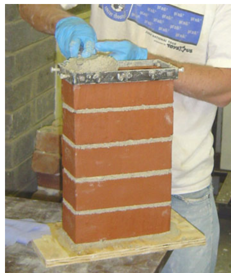
Fig. 1 Prism assembly with mortar joint template
