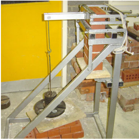
Fig. 2 Bond wrench testing apparatus
