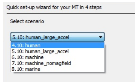
Figure 3. Different Xsens Kalman Filter-3 Scenarios for Various Testing Conditions
