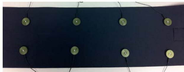
Figure 2. Four Columns and Two Rows of Tactors (4 columns by 2 rows)
