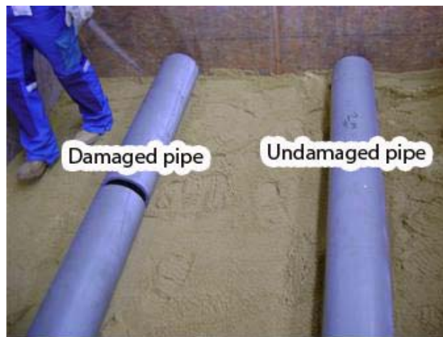
Figure 3.7: Arrangement of the two plastic pipes in the test box prior to burial
