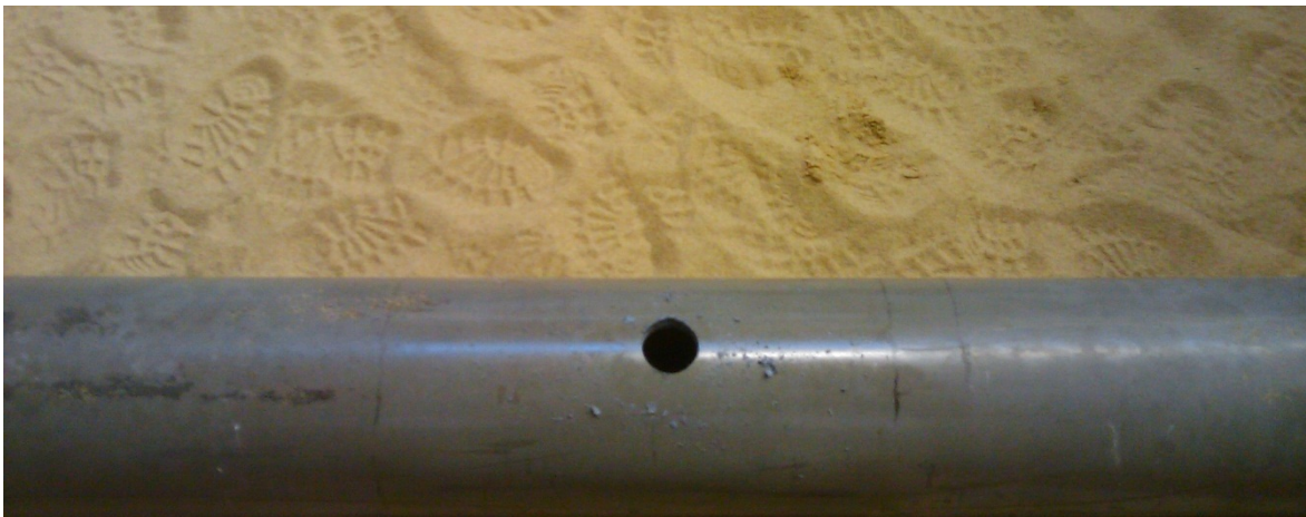
Figure 4.38: Test 3 –5cm hole in the pipe prior to being covered with sand
