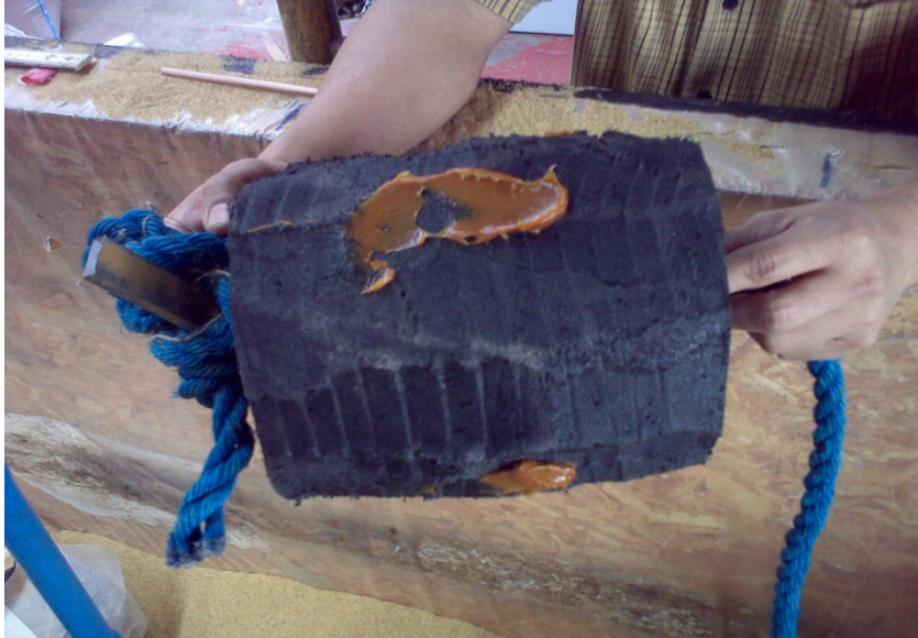
Figure 4.75. Test 7 - A sponge was used to block the hole in the pipe that could be subsequently removed
