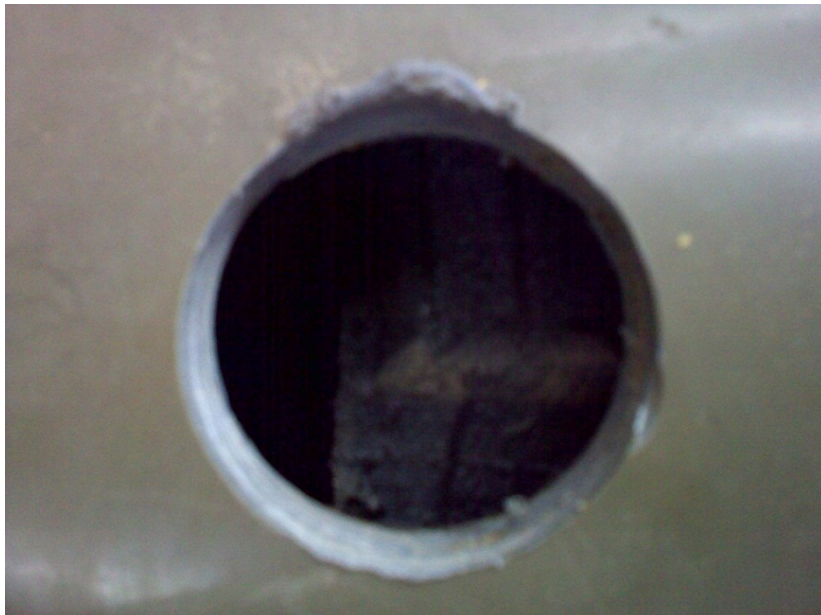
Figure 4.74: Test 7 - A 5cm diameter hole in the pipe
