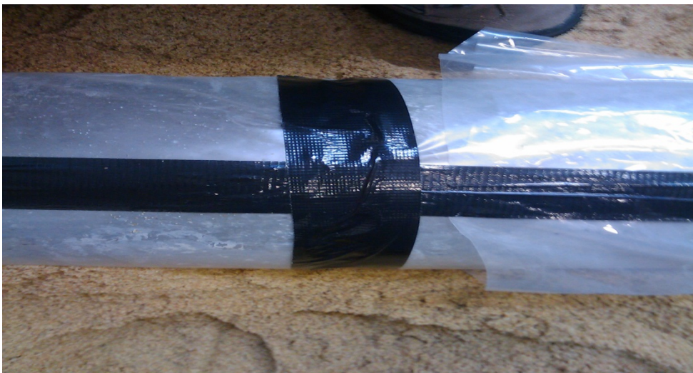
Figure 4.29. Test 2 - Broken pipe with a 2cm gap with a plastic cover
