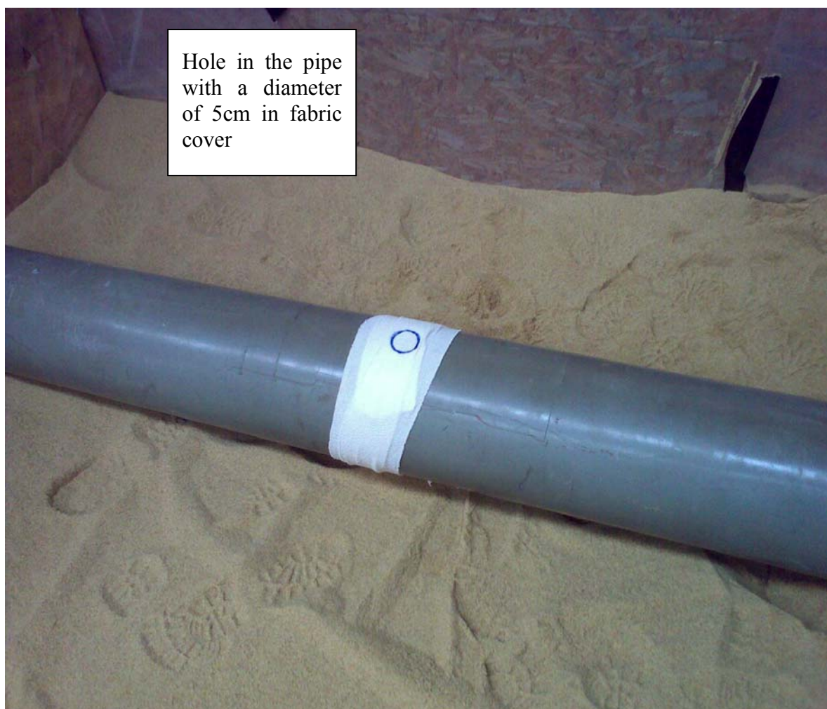
Figure 3.23: Hole in pipe with a diameter of 5cm gap in fabric cover
