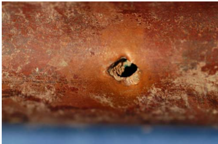
Figure 2.10: 10mm hole in metal pipe with 180 mm diameter
