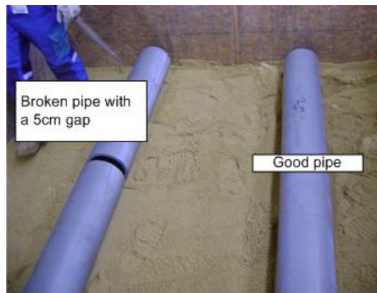
Figure 3.18: Test 1 during filling of the test facility
