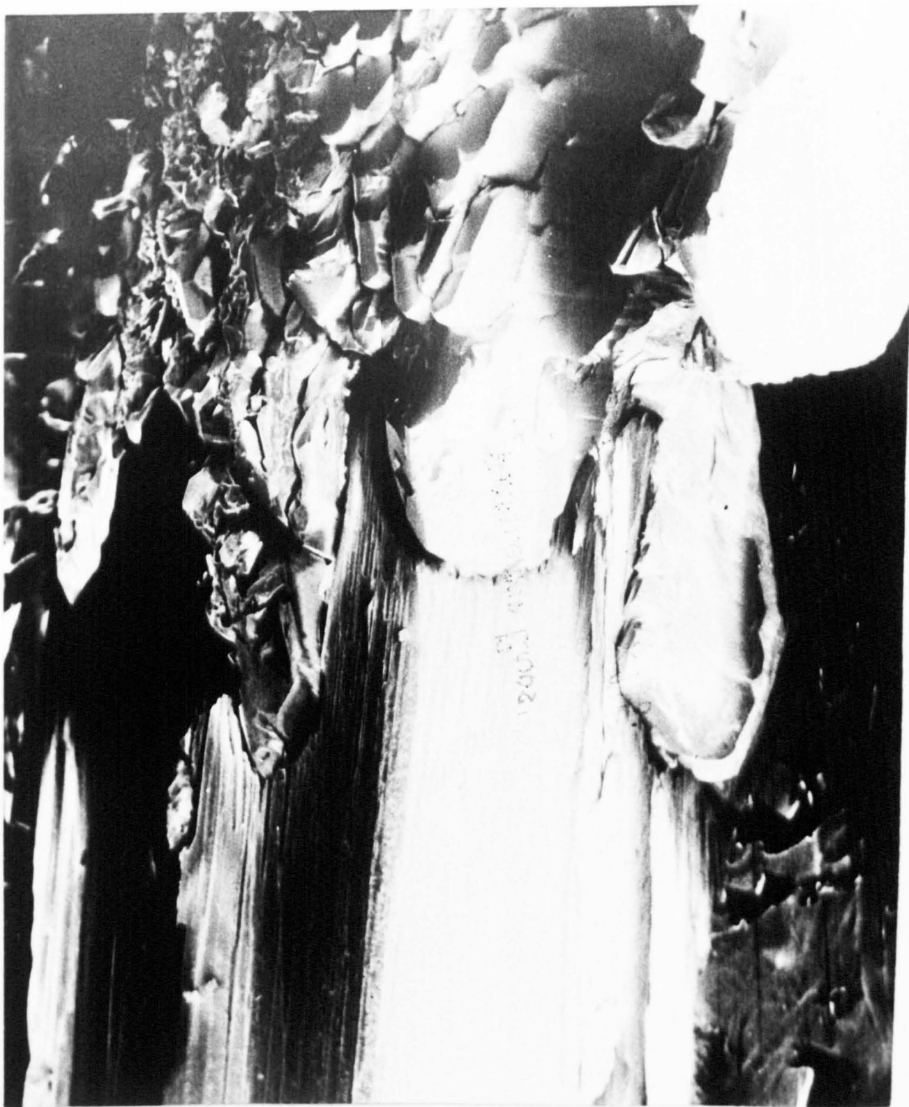
A view of MNA-1 crystals (upper) formed from MNA-3 (lower) in the solid phase at ambient temperature. (x 500)
