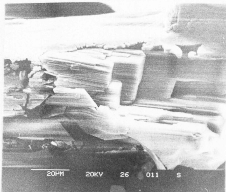
Tightly packed crystals of MNA-1 (right) formed from MNA-3(left) at ambient temperature in the solid phase. This represents 'vertical' growth of MNA-1 from MNA-3. The MNA-1 and MNA-3 axes are horizontal.
