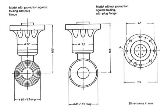
Figure 8.8.7. Specification and drawing of conductivity sensor (NSW, 1985).
