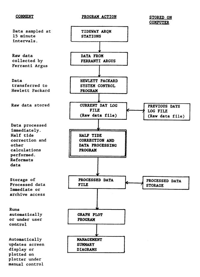
Figure 9.2.1. Data flow Diagram - Processing Method for tidal ARQM.
