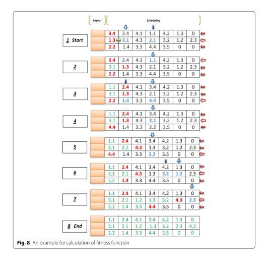
Step 4 The first, second and third steps are repeated until the completion times of all genes  $(CTM_{k'j})$  are obtained. Following these steps and considering the constraints (9) and (10), the  $(CTP_i)$  values and the makespan value  $(C_{max})$  are returned.
