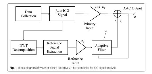
signal is constructed for any type of contamination present in the raw input ICG signal. The constructed reference signal is used as the reference signal for the adaptive algorithm to update its weight coefficients. The proposed AAC thus plays a vital role in the implementation of an intelligent remote health care monitoring system that is referencefree by constructing the reference signal itself from the contaminated input signal.
