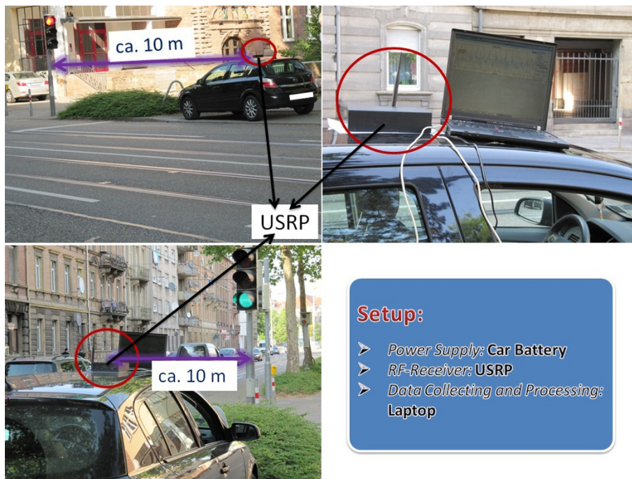
Figure 3 Experimental setup for the proposed traffic awareness system in the static situation.
