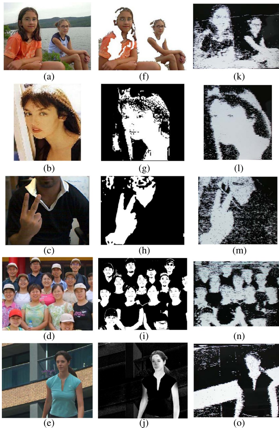
Figure 8 The comparison with skin detection methodologies from references; (a)-(e) are test scenarios from Table 2, (1)-(5) with their results in (f)-(j), and (k)-(o) are for pixel-based TCH tested without noise filter.
