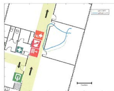
Figure 6: Estimated trajectory of the IMU post-calibration with and without applying loop-closure
