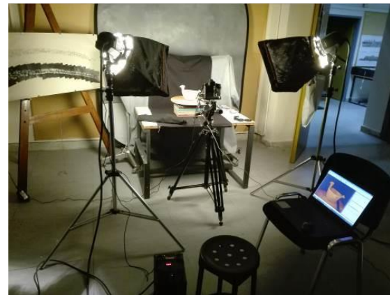
Figure 3: Focus stacking acquisition set-up
