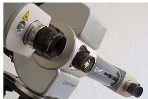
Figure 1: SmartSCAN 3D-HE structured light system (Breuckmann, 2017)
