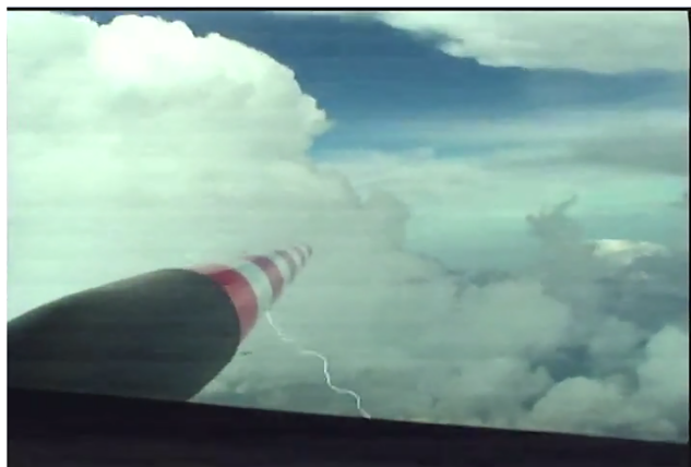
Figure 6. Image taken from the HALO cockpit just before the aircraft penetration of a convective cloud with lightning activity during flight AC07. In this case, the cloud pass height was 9022 m (temperature \sim -25^\circ\text{C} ) and the maximum CWC measured was 0.55\text{ g m}^{-3} .
