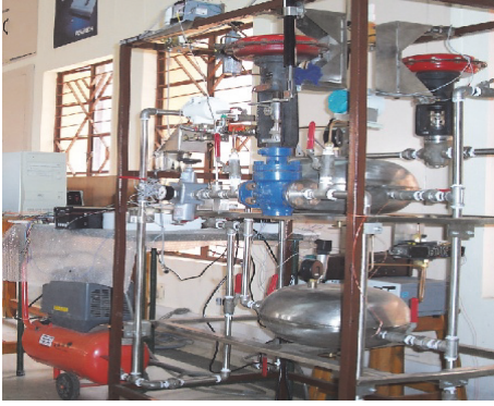
FIGURE 1: Photograph of the pneumatic pressure system.
