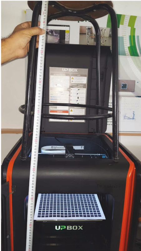
FIGURE 11: The camera calibration test setup. Using a calibrated 3D printer with a robotic moving panel, we were able to calibrate the Z approximation up to the 0.4 mm accuracy level.
