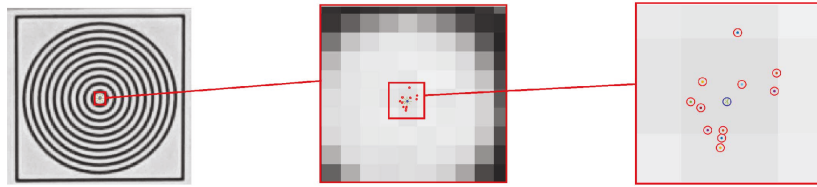
FIGURE 6: An example of the K -means clustering (KMC) result; the dotted points on the right are the centers of the ellipses, and the starred ones (blue) are the KMC result.
