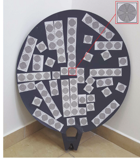
FIGURE 4: The multicircular targets on a solid main reflector as acquired by the moncamera.
