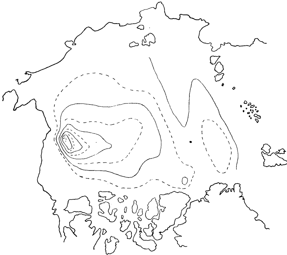
FIG. 11. Streamline pattern for the wind-driven case after 600 days. Non-linear terms, bottom and lateral friction, inflow-outflow on the boundaries, and 10% of the bathymetric variation are included. Between solid lines the transport is 10^7 \text{ m}^3 \text{ sec}^{-1} .
