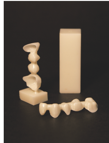
FIGURE 1: Right. Zirconia blank. Left. Direct from machining of FDP framework. Front. Zirconia FDP framework designed using a CAD program, ready for veneering (Denzir, Cad.esthetics AB, Skellefteå, Sweden).
