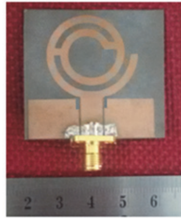
FIGURE 11: Prototype of antenna fabricated on Rogers RT/duroid 5880 substrate.
