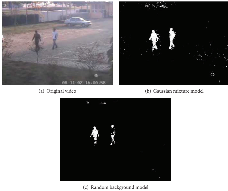
FIGURE 3: The target detection results of video data 2.
