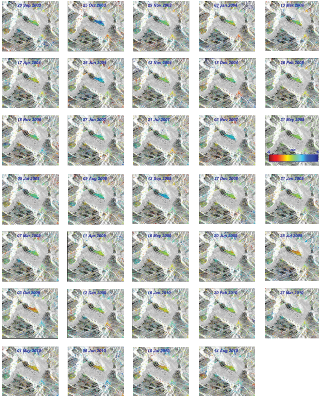
FIGURE 8: Time series of LOS deformation at Hanyuan spanning from September 2003 to August 2010, referenced temporally to the “master” scene (May 31, 2008) and superimposed on the mean amplitude image.
